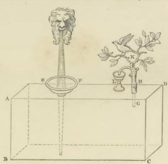
will be that the air, being driven out, passes through the pipe GHK, and emits a sound. When the extremity of the pipe dips into water a bub-
